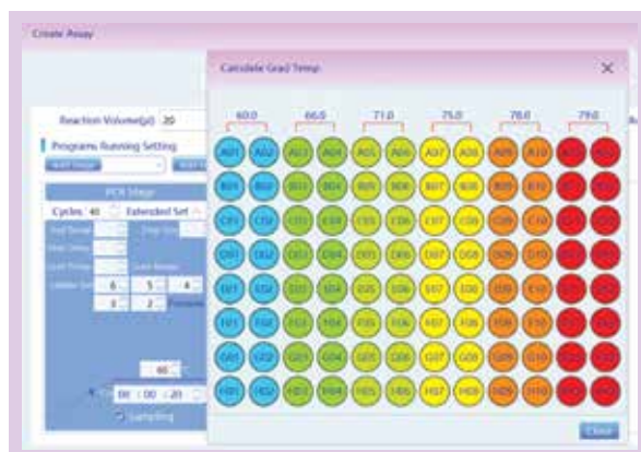
Figure 2: Thermal Gradient for Insta Q96® AG series
