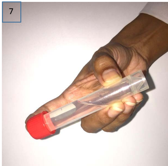
7 Tilt the tubes in upside down position for proper mixing
