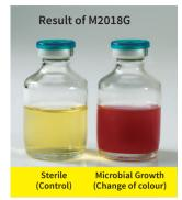
Media fills simulate the whole process in order to evaluate the sterility confidence of the process. Process simulation studies include formulation, filtration and filling with suitable media. In general, a microbiological growth medium such as Tryptic Soy Broth should be used. Use of anaerobic growth media (e.g. Fluid Thioglycollate medium) should be considered in special circumstances.
