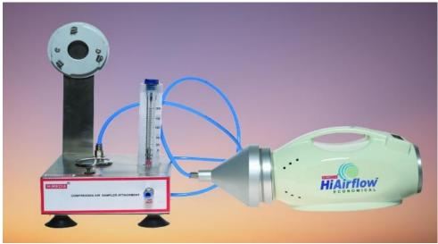
HiMedia Compressed Air Sampler (diffuser) with LA881HiAirflow Economical to test the quality of compressed air and gases used in cleanrooms. A compressed air source is connected and the flow meter regulated to achieve the required flow rate.
